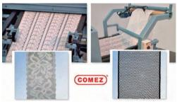
the stretched fabric into a heated chamber, where the combined action of heat and ventilation quickly fixes its dimension. The fabric speed can be varied according to the type of fabrics.
